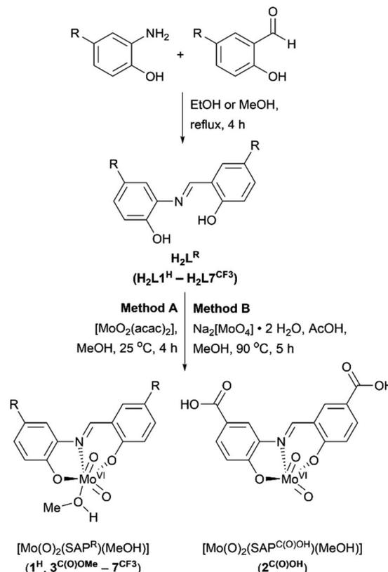
Scheme 3 Synthesis of SAP-type ligands ( $H_2L^R$ ) and  $cis$ - $Mo^{VI}(O)_2$  complexes ( $1^{H-7CF_3}$ ). Where R = H ( $H_2L1^H$  and  $1^H$ );  $C(O)OH$  ( $H_2L2^{C(O)OH}$  and  $2^{C(O)OH}$ );  $C(O)OMe$  ( $H_2L3^{C(O)OMe}$  and  $3^{C(O)OMe}$ ); F ( $H_2L4^F$  and  $4^F$ ); tBu ( $H_2L5^{tBu}$  and  $5^{tBu}$ ); OMe ( $H_2L6^{OMe}$  and  $6^{OMe}$ );  $CF_3$  ( $H_2L7^{CF_3}$  and  $7^{CF_3}$ ).
