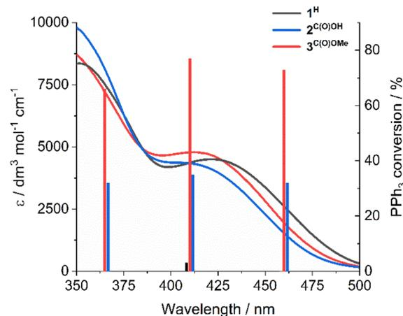
Fig. 3 UV-vis spectra of  $1^{\text{H}}$ ,  $2^{\text{C(O)OH}}$ , and  $3^{\text{C(O)OMe}}$  and  $\text{PPh}_3$  conversion as a function of irradiation wavelength. Photocatalytic conditions: catalyst (1 mM in  $\text{DMSO-d}_6$ ), 300 equivalents  $\text{PPh}_3$ , 3 h, under  $\text{N}_2$ .
