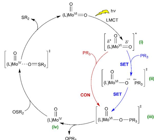
Scheme 5 Proposed catalytic mechanisms for light-activated OAT between phosphine and sulfoxide substrates, catalysed by photoactive *cis*- $\text{Mo}^{\text{VI}}(\text{O})_2$  complexes (SET = single electron transfer, CON = concerted reaction, comproportionation as shown in Scheme 4 also conceivable).
