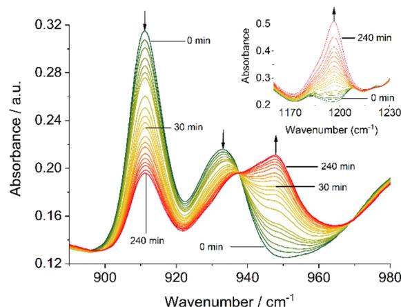
Fig. 4 Solution-IR spectra in the region of the Mo=O stretching bands ( $890\text{--}900\text{ cm}^{-1}$ ) of  $3^{\text{C(O)OMe}}$  (50 mM in DMF), 10 equivalents  $\text{PPh}_3$  and 50 equivalents  $\text{DMSO-d}_6$  in DMF irradiated at  $410\text{ nm}$  as a function of time; insert—O=P stretching band ( $1160\text{--}1230\text{ cm}^{-1}$ ) of the same sample.
