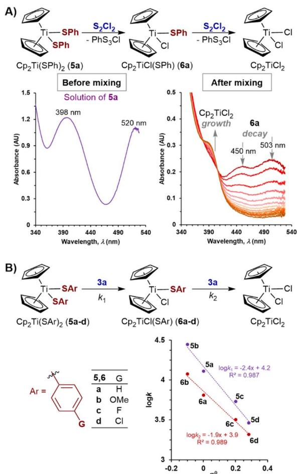
Fig. 6 (A) SF-UV monitoring of the reaction of titanocene bithiophenolate **5a** with  $S_2Cl_2$  at 22 °C. (B) Yukawa–Tsuno linear free energy correlation for thiophenolates **5a–d** and **6a–d** in reaction with **3a**.
