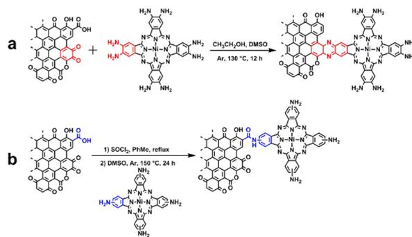
Scheme 1 Synthesis of (a) Ni(NH<sub>2</sub>)<sub>8</sub>Pc-GC and (b) Ni(NH<sub>2</sub>)<sub>4</sub>Pc-GC.
