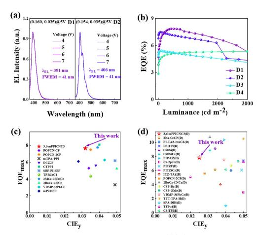
Fig. 7 (a) Normalized EL spectra at different applied voltages of the devices **D1** and **D2**. (b) EQE *versus* luminance curves of the devices **D1**–4. EQE<sub>max</sub> *versus* CIEy of the reported non-doped (c) and doped (d) HLCT-based OLEDs with a CIEy value below 0.05.
