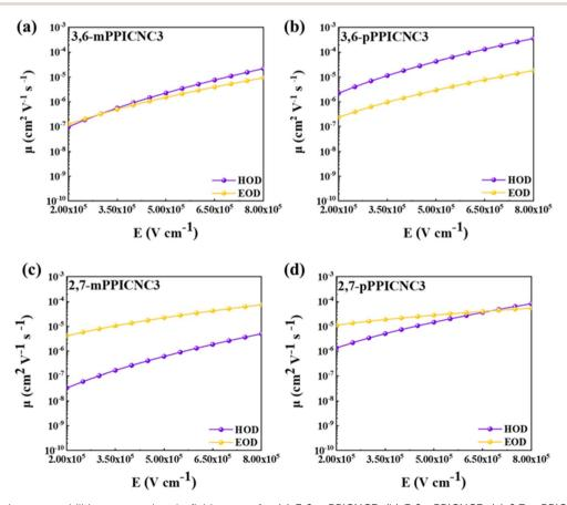
Fig. 5 Hole and electron mobilities *versus* electric field curves for (a) 3,6-mPPICNC3, (b) 3,6-pPPICNC3, (c) 2,7-mPPICNC3 and (d) 2,7-pPPICNC3.
