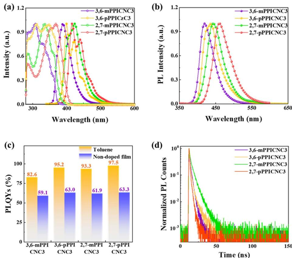
Fig. 3 (a) Normalized absorption and PL spectra of 3,6-mPPICNC3, 3,6-pPPICNC3, 2,7-mPPICNC3 and 2,7-pPPICNC3 in toluene solution (10<sup>-5</sup> M). (b) Normalized PL spectra in the neat film. (c) PLQYs in toluene and the neat film. (d) Transient PL decay spectra in the neat film.
