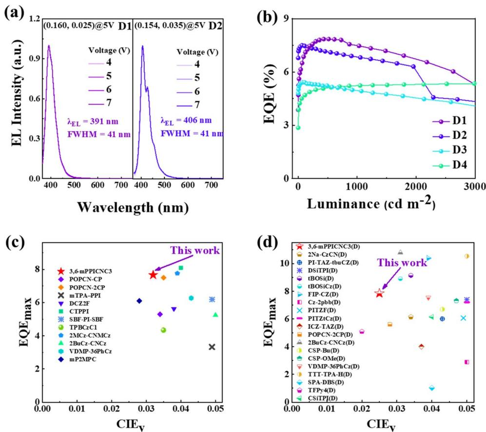
Fig. 7 (a) Normalized EL spectra at different applied voltages of the devices D1 and D2. (b) EQE versus luminance curves of the devices D1–4. EQE<sub>max</sub> versus CIE<sub>y</sub> of the reported non-doped (c) and doped (d) HLCT-based OLEDs with a CIE<sub>y</sub> value below 0.05.
