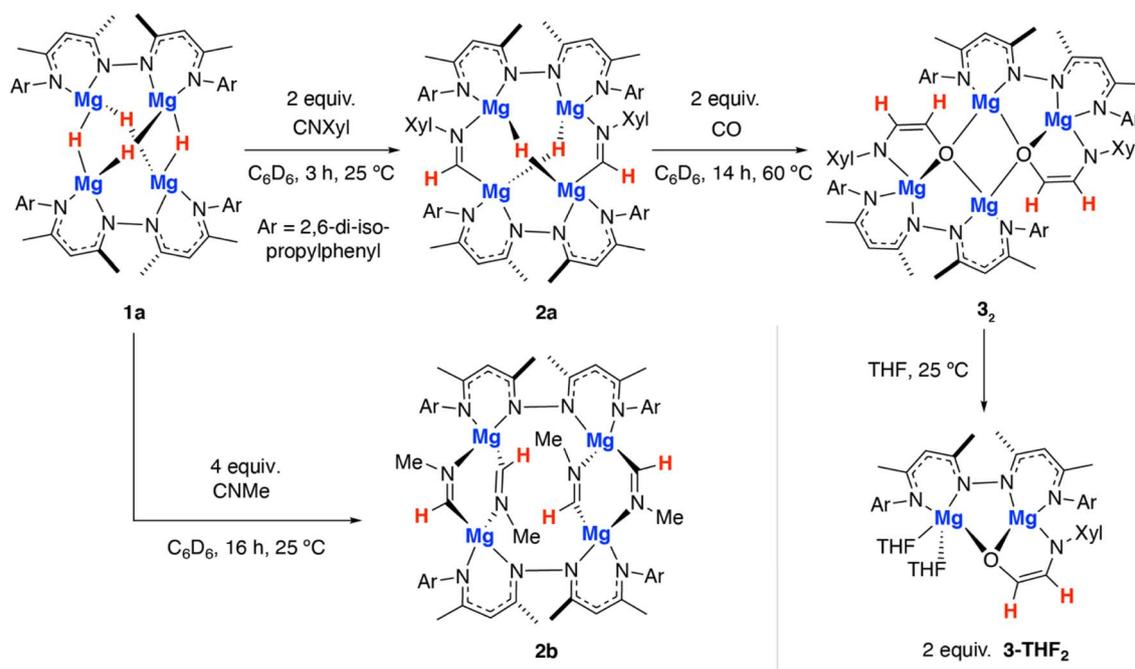
Scheme 1 Reactions of a tetrametallic magnesium hydride cluster **1a** with isocyanides and CO.
