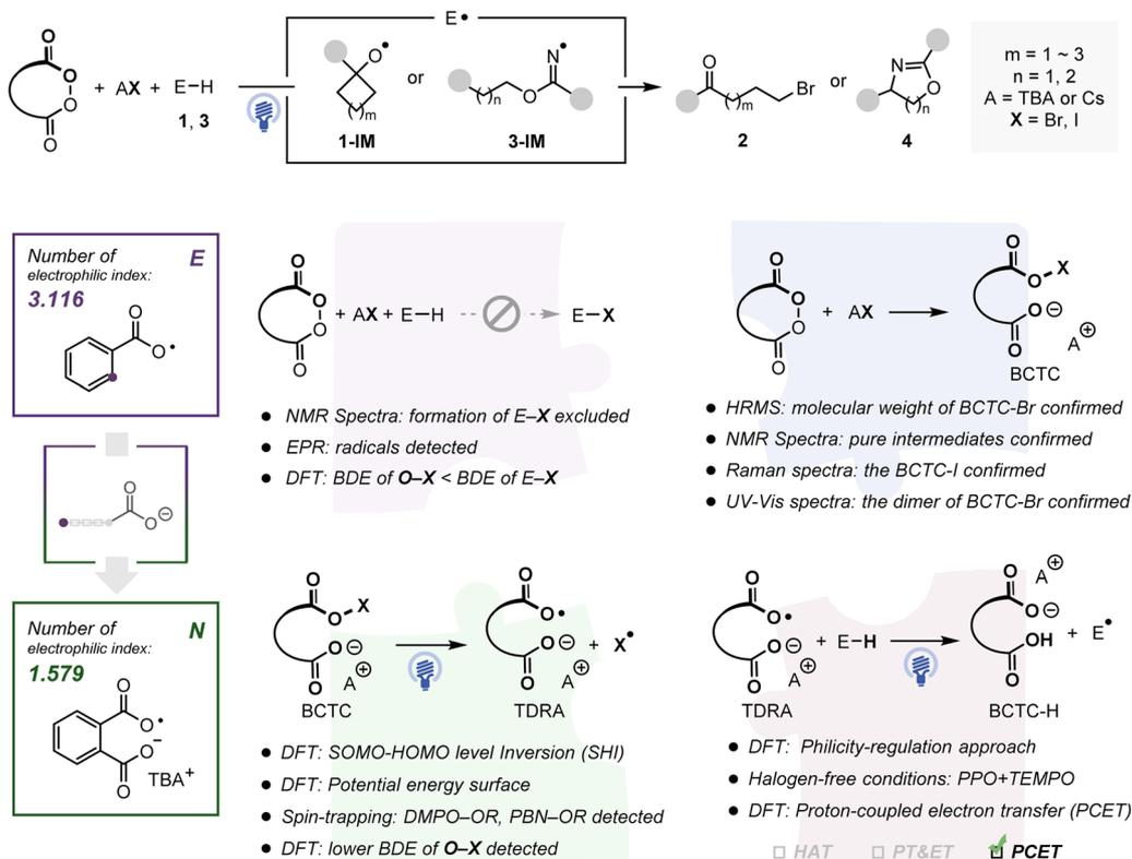
Fig. 1 (a) Strategies for the indirect generation of heteroatom-centered radicals. (b) Strategies for the direct generation of heteroatom-centered radicals. (c) Critical experimental and theoretical studies for the TDRA-mediated generation of heteroatom-centered radicals through the philicity-regulation approach and PCET step.
