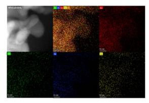
Fig. 4 HAADF-STEM image and corresponding EDS mapping images of the fresh KFeCuZn/ZrO2 that has undergone calcination at 500 °C under air.
