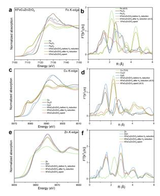
Fig. 3 Ex situ XAS spectra of KFeCuZn/ZrO $_2$  before and after H $_2$  reduction at 400 °C as a pretreatment and after reaction (spent). (a) Normalized Fe K-edge XANES spectra; (b) FT-EXAFS spectra for Fe; (c) normalized Cu K-edge XANES spectra; (d) FT-EXAFS spectra for Cu; (e) normalized Zn K-edge XANES spectra; and (f) FT-EXAFS spectra for Zn. "Spent catalyst" refers to a sample that has undergone a 20 hours accelerated aging treatment at 400 °C under the reaction condition.
