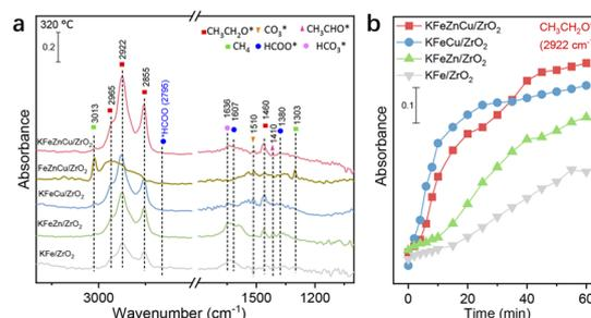
Fig. 8 *In situ* DRIFTS spectra. (a) Different catalysts under the  $\text{CO}_2 + \text{H}_2$  reaction after 60 min at 320 °C and 0.5 MPa; (b) dynamic IR peak intensities of  $\text{CH}_3\text{CH}_2\text{O}^*$  ( $2922 \text{ cm}^{-1}$ ) at 320 °C for different catalysts.
