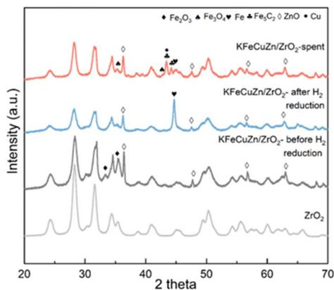
Fig. 2 XRD patterns of KFeCuZn/ZrO<sub>2</sub> before and after H<sub>2</sub> reduction at 400 °C as a pretreatment and after reaction. "Spent catalyst" refers to a sample that has undergone a 20 hours accelerated aging treatment at 400 °C under the reaction conditions.
