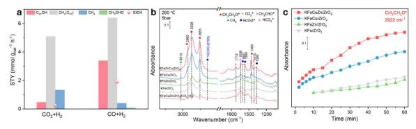
Fig. 10 (a) Catalytic performance over the KFeCuZn/ZrO $_2$  catalyst under a CO/H $_2$  or CO $_2$ /H $_2$  flow at 280 °C and 3 MPa; (b) *in situ* DRIFTS spectra of the CO + H $_2$  reaction over the different catalysts under a CO/H $_2$  flow at 280 °C and 0.5 MPa; and (c) dynamic IR peak intensities of CH $_3$ CH $_2$ O\* (2922 cm $^{-1}$ ) at 280 °C.
