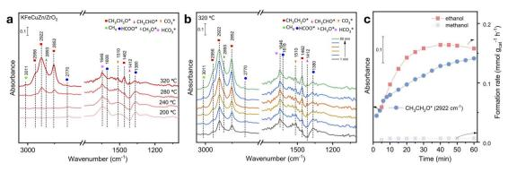
Fig. 7 In situ/operando DRIFTS spectra. (a) DRIFTS spectra of the  $CO_2 + H_2$  reaction over KFeCuZn/Zr $O_2$  after 60 min at 0.5 MPa and different temperatures; (b) time resolution spectra of the  $CO_2 + H_2$  reaction over KFeCuZn/Zr $O_2$  at 0.5 MPa and 320 °C; (c) dynamic IR peak intensities of  $CH_3CH_2O^*$  (2922 cm<sup>-1</sup>) and formation rate of ethanol and methanol, quantified by micro-GC at 320 °C.
