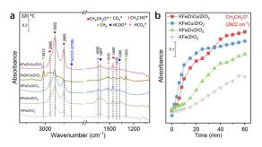
Fig. 8 In situ DRIFTS spectra. (a) Different catalysts under the  $CO_2$  +  $H_2$  reaction after 60 min at 320 °C and 0.5 MPa; (b) dynamic IR peak intensities of  $CH_3CH_2O^*$  (2922 cm $^{-1}$ ) at 320 °C for different catalysts.
