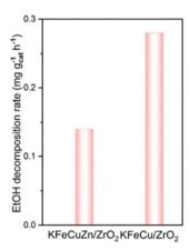
Fig. 9 EtOH decomposition over the KFeCuZn/ZrO $_2$  and KFeCu/ZrO $_2$  catalysts (conditions: batch reactor, spent catalysts: 50 mg, N $_2$ : 0.5 MPa, at 260 °C, 3 h, ethanol (0.3 mL) + octane (0.7 mL)).
