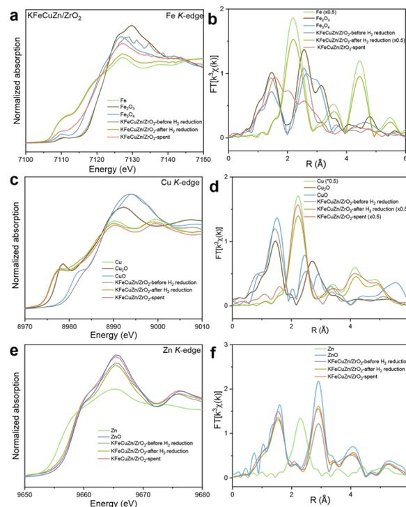
Fig. 3 *Ex situ* XAS spectra of KFeCuZn/ZrO<sub>2</sub> before and after H<sub>2</sub> reduction at 400 °C as a pretreatment and after reaction (spent). (a) Normalized Fe K-edge XANES spectra; (b) FT-EXAFS spectra for Fe; (c) normalized Cu K-edge XANES spectra; (d) FT-EXAFS spectra for Cu; (e) normalized Zn K-edge XANES spectra; and (f) FT-EXAFS spectra for Zn. "Spent catalyst" refers to a sample that has undergone a 20 hours accelerated aging treatment at 400 °C under the reaction condition.
