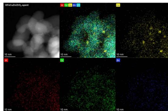
Fig. 5 HAADF-STEM image and corresponding EDS mapping images of the spent KFeCuZn/ZrO<sub>2</sub> that has undergone a 20 hours accelerated aging treatment at 400 °C under the reaction condition.
