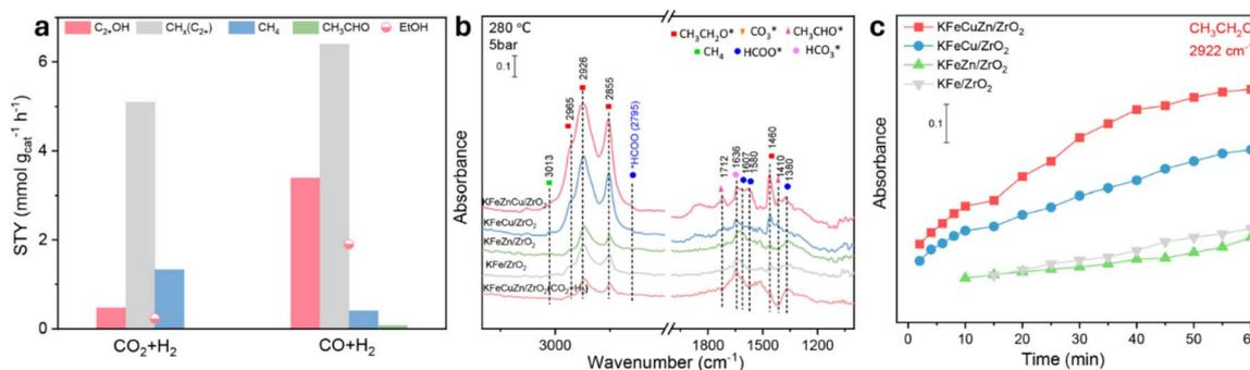
Fig. 10 (a) Catalytic performance over the KFeCuZn/ZrO<sub>2</sub> catalyst under a CO<sub>2</sub>/H<sub>2</sub> or CO/H<sub>2</sub> flow at 280 °C and 3 MPa; (b) *in situ* DRIFTS spectra of the CO + H<sub>2</sub> reaction over the different catalysts under a CO/H<sub>2</sub> flow at 280 °C and 0.5 MPa; and (c) dynamic IR peak intensities of CH<sub>3</sub>CH<sub>2</sub>O\* (2922 cm<sup>-1</sup>) at 280 °C.
