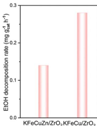
Fig. 9 EtOH decomposition over the KFeCuZn/ZrO<sub>2</sub> and KFeCu/ZrO<sub>2</sub> catalysts (conditions: batch reactor, spent catalysts: 50 mg, N<sub>2</sub>: 0.5 MPa, at 260 °C, 3 h, ethanol (0.3 mL) + octane (0.7 mL)).
