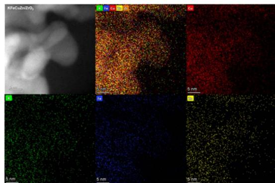
Fig. 4 HAADF-STEM image and corresponding EDS mapping images of the fresh KFeCuZn/ZrO<sub>2</sub> that has undergone calcination at 500 °C under air.
