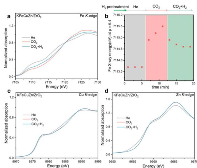
Fig. 6 *In situ* XAFS spectra of KFeCuZn/ZrO<sub>2</sub>. (a) Normalized Fe K-edge XANES spectra; (b) X-ray energy at normalized absorption ( $\mu = 0.4$ ) under different atmospheres; (c) Cu K-edge XANES spectra; and (d) Zn K-edge XANES spectra. Conditions: 400 °C and 1 bar.
