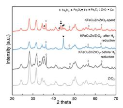
Fig. 2 XRD patterns of KFeCuZn/ZrO $_2$  before and after H $_2$  reduction at 400 °C as a pretreatment and after reaction. "Spent catalyst" refers to a sample that has undergone a 20 hours accelerated aging treatment at 400 °C under the reaction conditions.
