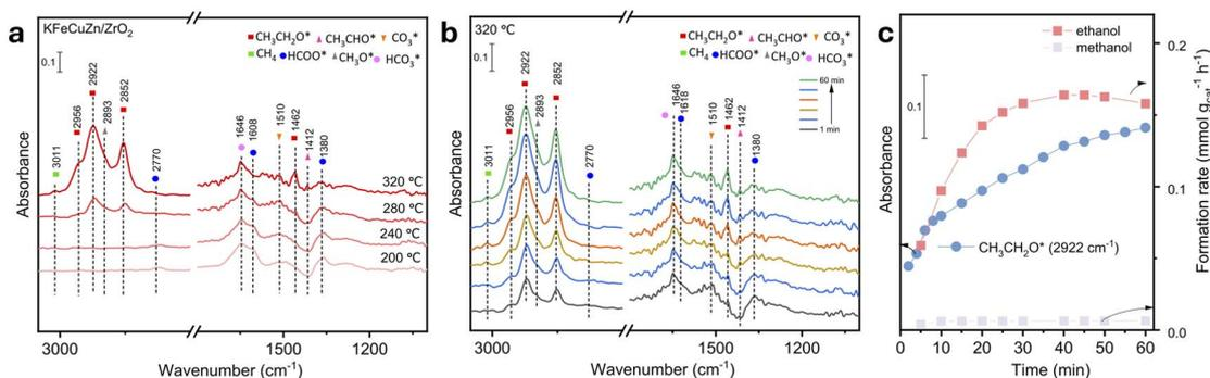
Fig. 7 *In situ/operando* DRIFTS spectra. (a) DRIFTS spectra of the  $\text{CO}_2 + \text{H}_2$  reaction over  $\text{KFeCuZn/ZrO}_2$  after 60 min at 0.5 MPa and different temperatures; (b) time resolution spectra of the  $\text{CO}_2 + \text{H}_2$  reaction over  $\text{KFeCuZn/ZrO}_2$  at 0.5 MPa and 320 °C; (c) dynamic IR peak intensities of  $\text{CH}_3\text{CH}_2\text{O}^*$  ( $2922 \text{ cm}^{-1}$ ) and formation rate of ethanol and methanol, quantified by micro-GC at 320 °C.
