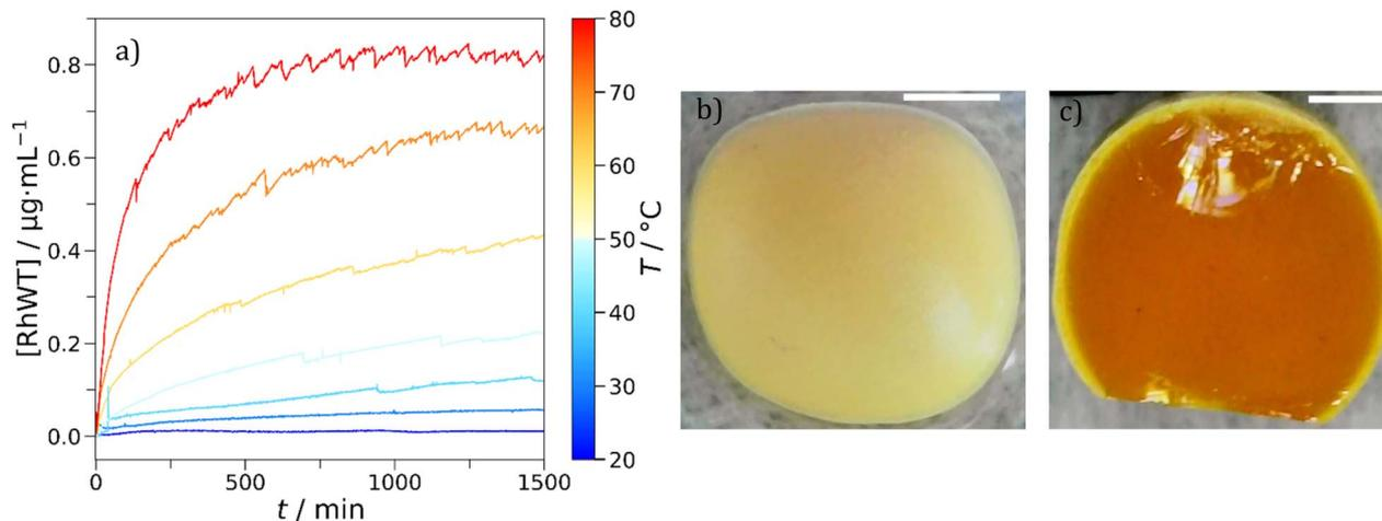
Fig. 7 (a) Release of rhodamine WT (RhWT) from Cha/Bif glass, measured as a function of temperature ( $T$ ) and time ( $t$ ) using UV-vis absorbance spectroscopy (556 nm). (b) A different Cha/Bif particle after being submerged in water for a week. (c) Cross-section of the opaque Cha/Bif particle. The opaque crystalline shell is approximately 150  $\mu\text{m}$  thick. The inner core remains as it were at  $t_0$ . Scale bars: 1 mm.
