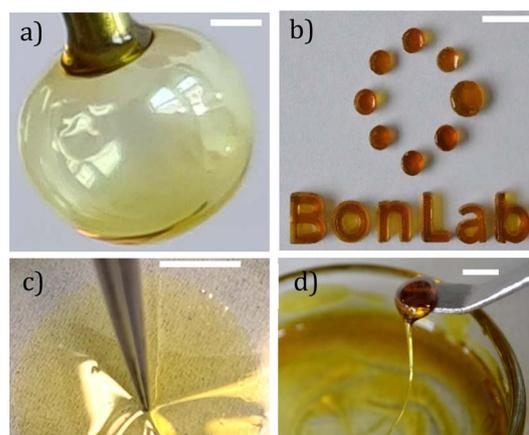
Fig. 5 (a) Bubble of Cha/Bif eutectic glass. (b) Molding of Cha/Bif into complex shapes. (c) Formation of a Cha/Bif glass film by deposition from EtOAc (33.9 mg g<sup>-1</sup>) partitioned above EtOAc-saturated water. Flexibility is demonstrated by physical deformation. (d) Pulling of a Cha/Bif glass fiber. Scale bars = 1 mm (a–c) and 5 mm (d).
