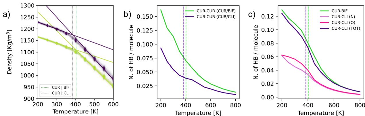
Fig. 3 (a) Computational estimate of the  $T_g$  of the Cur/Bif ( $403 \pm 6$  K, green vertical line) and Cur/Cli ( $385 \pm 5$ , purple vertical line) mixtures. (b) Number of curcumin–curcumin hydrogen bonds (per molecule) for the Cur/Bif and Cur/Cli mixture as a function of temperature. (c) Number of curcumin–bifonazole/climbazole hydrogen bonds (per molecule) for the Cur/Bif and Cur/Cli mixture as a function of temperature.
