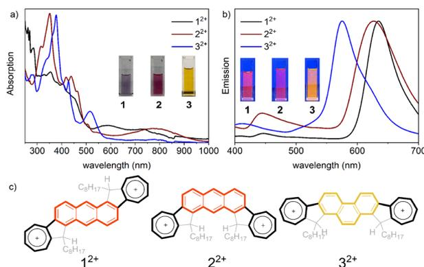
Fig. 6 Protonation behaviour: (a) UV-vis absorption and (b) emission of protonated compounds **1**<sup>2+</sup>, **2**<sup>2+</sup>, and **3**<sup>2+</sup>. Insets show photos of the solutions. (c) The structure of protonated compounds.
