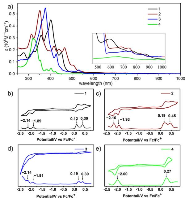
Fig. 4 (a) UV-vis absorption ( $10^{-6}$  M in DCM). Cyclic voltammetry (CV) curves and differential pulse voltammetry (DPV) curves of (b) **1**, (c) **2**, (d) **3**, and (e) **4**, measured in 0.1 M solution of  $^n\text{Bu}_4\text{NPF}_6$  in DCM.
