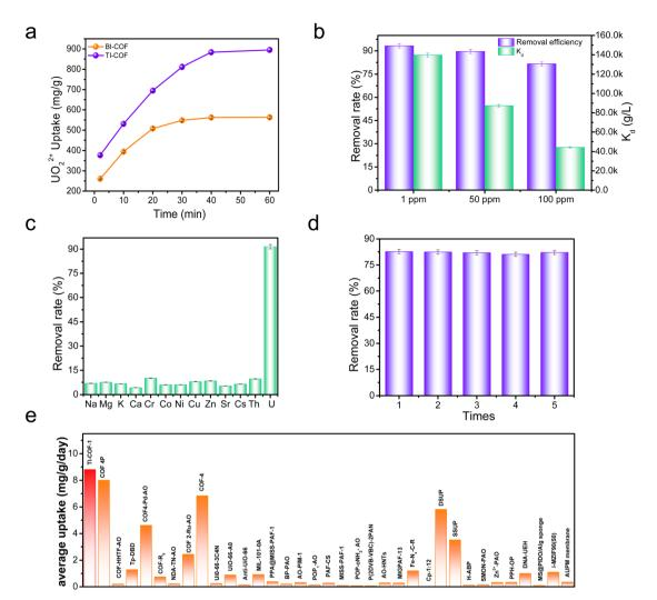
(a) Uranium extraction kinetics upon the BI-COF and TI-COF for a 50 mL 100 ppm U solution. (b) A comparison of the removal rate and  $K_d$ value for the TI-COF in 100, 50, and 1 ppm U solutions. (c) Selective extraction towards U over other ions. (d) Recycle of TI-COF. (e) A comparison of uranium extraction efficiency among reported adsorbents and our case. The error bars are based on the average value of three times.
