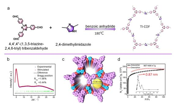
Fig. 2 (a) Synthesis route of the TI-COF. (b) Experimental PXRD pattern and Pawley refinement. (c) View of the staggered (AB) stacking structure with a 1D channel. (d)  $N_2$  adsorption—desorption isotherms at 77 K with the inset of pore size distribution.
