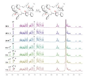
Fig. 1 NMR deuterium exchange in cobalt( $_{\rm III}$ ) metallohelices. The imine deuterium exchange of  $\Lambda$ -6 monitored by  $^{\rm 1}$ H NMR spectroscopy (400 MHz, 298 K, D $_{\rm 2}$ O).
