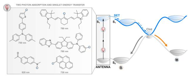
Fig. 2 Two-photon excitation of a covalently linked absorber (antenna), subsequent singlet energy transfer to the photoswitch, and the following events in the excited state.
