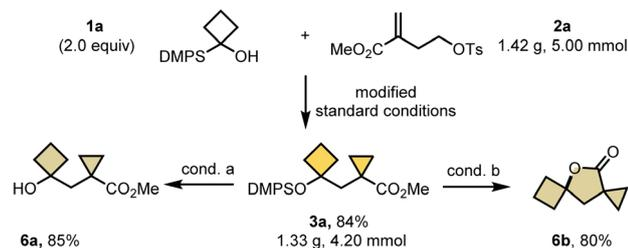
**Scheme 3** Scale-up reaction and follow-up chemistry. Isolated yields are shown; conditions for **6a**: *n*-Bu<sub>4</sub>NF (2.5 equiv.), NaF (3.0 equiv.), THF/MeOH, rt, 6 h; conditions for **6b**: *n*-Bu<sub>4</sub>NF (5.0 equiv.), dry DCM, rt, 10 min. See ESI† for details.
