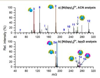
Fig. 2 Ex situ nano-DESI MS of the deposition spots of  $[Ni(bpy)_3]^{2+}$  analyzed with (a) ACN and (b) 3  $\mu$ M bpyD in ACN as the nano-DESI solvent. Ion assignments are listed in Table 1. The pictograms symbolize the number of ligands coordinated to Ni. Green and pink symbols represent bpy and bpyD, respectively. Peaks originating from the solvent are not marked in the spectra for simplicity.
