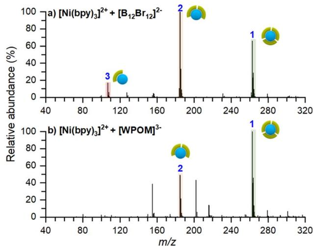
Fig. 6 *Ex situ* MS of surfaces prepared by co-depositing  $[\text{Ni}(\text{bpy})_3]^{2+}$  with (a)  $[\text{B}_{12}\text{Br}_{12}]^{2-}$ , and (b)  $[\text{WPOM}]^{3-}$ . Both surfaces show an increased abundance of  $[\text{Ni}(\text{bpy})_3]^{2+}$  and only minor products of dissociation.
