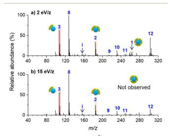
Fig. 3 Ex situ mass spectra of  $[Ni(bpy)_3]^{2+}$  deposited at (a) 2 eV/z and (b) 15 eV/z.
