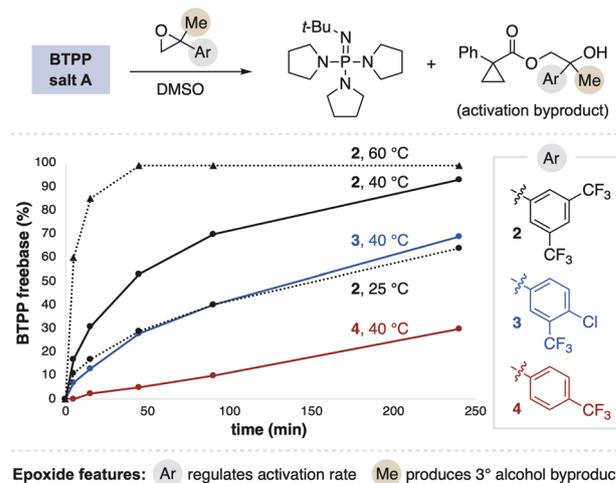
Fig. 3 (a) Synthesis and (b) activation of BTTP salt A. <sup>a</sup> Activation studies run with 1 equiv BTTP salt A and 2 equiv epoxide; all conditions ultimately reach near-complete BTTP generation. See ESI† for details on data collection and analysis.
