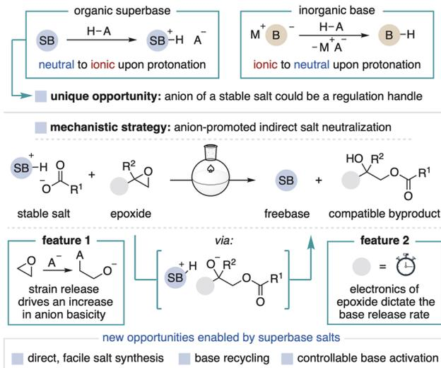
Fig. 2 Mechanistic design for superbase precatalyst system.
