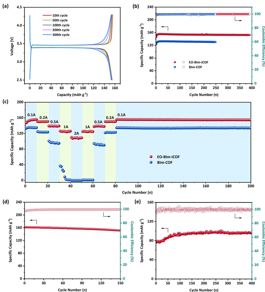
Fig. 4 (a) The voltage profiles, (b) cycling stability and coulombic efficiency of the LFP||LITFSI@EO-BIm-iCOF||Li cell at 100 mA g<sup>-1</sup>. (c) Rate capabilities of the LFP||LITFSI@COFs||Li cells. (d) Cycling stability and coulombic efficiency of the LFP||LITFSI@EO-BIm-iCOF||Li cell at 100 mA g<sup>-1</sup> at 60 °C. (e) Cycling stability and coulombic efficiency of the LFP||LITFSI@EO-BIm-iCOF||Li cell at 50 mA g<sup>-1</sup> at -10 °C.
