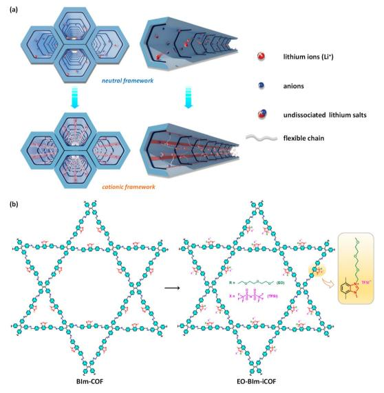
Fig. 1 (a) Schematic illustration of the lithium ion transport process in COFs with the traditional bare channels and integrated "rigid-flexible" strategy, respectively. (b) Synthetic scheme of the two-dimensional mesoporous BIm-COF and post-modified EO-BIm-iCOF, respectively.
