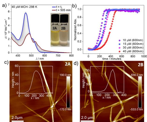
Fig. 2 (a) Time-dependent evolution of assembly **2A** into **2B** in MCH ( $c = 4 \times 10^{-5}$  M) at 298 K. (b) Plot of absorbance vs. time at  $\lambda = 600$  nm using different concentrations ( $c = 10$ – $40 \mu\text{M}$ ) at 298 K. AFM images of **2A** (c) and **2B** (d) obtained upon drop-casting the corresponding solutions ( $c = 1 \times 10^{-5}$  M) on HOPG.
