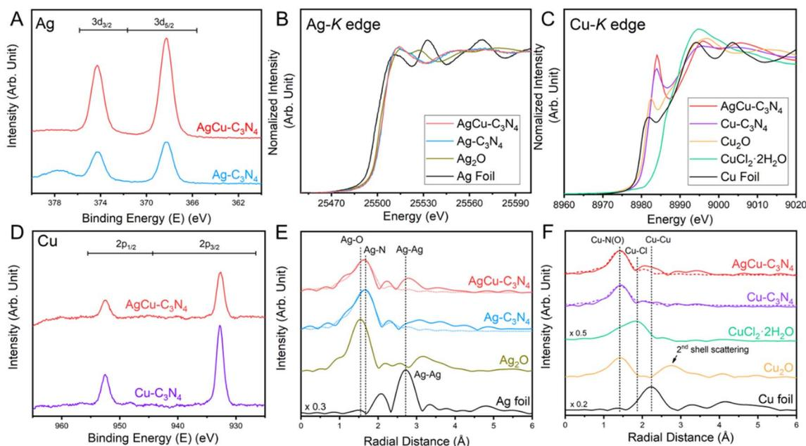
Fig. 2 Electronic structure of AgCu– $\text{C}_3\text{N}_4$  SAC. (A) Ag<sub>3d</sub> XPS, (B) Ag K-edge XANES spectra, (C) Cu K-edge XANES spectra, (D) Cu<sub>2p</sub> XPS, (E) Ag and (F) Cu FT-EXAFS spectra of AgCu– $\text{C}_3\text{N}_4$  SACs. The dotted lines represent the FT-fitting curves.
