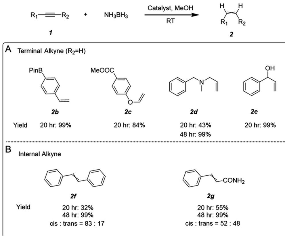
Fig. 4 The substrate scope of the  $\text{AgCu-C}_3\text{N}_4$  SAC catalysed alkyne semi-hydrogenation. (A) Multifunctional terminal aliphatic alkyne and aryl alkynes containing borate, amine, hydroxyl groups, and (B) internal alkynes can be processed with  $\text{AgCu-C}_3\text{N}_4$  SAC.
