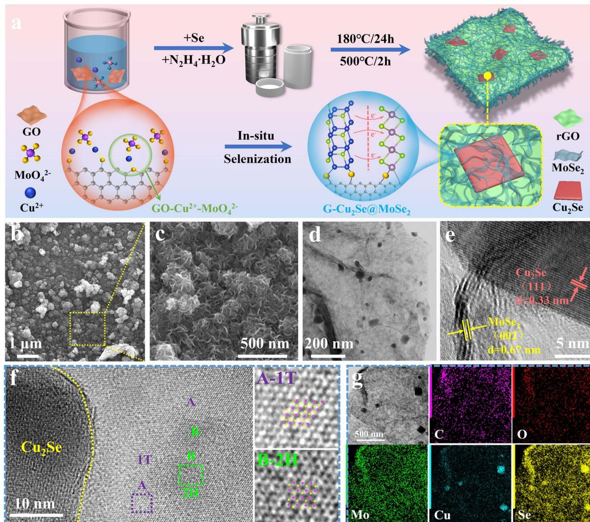
Fig. 2 Morphology of the heterogeneous G-Cu<sub>2</sub>Se@MoSe<sub>2</sub> composite. (a) Preparation procedures of the G-Cu<sub>2</sub>Se@MoSe<sub>2</sub> heterogeneous composite (schematic). (b and c) SEM images showing surface morphologies. TEM (d) and HRTEM (e and f) images. (g) EDS mapping images displaying the distribution of C, O, Mo, Cu and Se elements.
