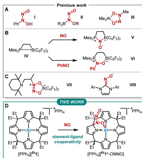
Fig. 1 (A–C) Previously reported reactivities of NO and nitrosobenzene with main-group element compounds. (D) Reactivity of calix[4]pyrrolato aluminate ([<sup>Et1</sup>]<sup>−</sup>) with NO studied within this work. The asterisk in [<sup>Et1</sup>\*-ONNO]<sup>−</sup> indicates the dearomatization of one pyrrole unit.
