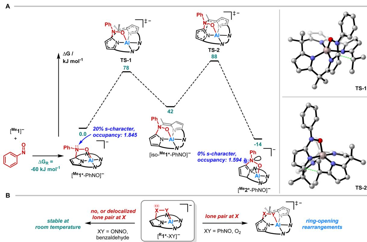
Fig. 5 (A) Computed reaction profile for the rearrangement of  $[\text{PPh}_4][\text{Me}1^*\text{-PhNO}]$  at the RI-DSD-PBEB95-D3(BJ)/def2-QZVPP, COSMO-RS( $\text{CH}_2\text{Cl}_2$ )/PBEh-3c level of theory and the respective transition structures. (B) Schematic representation on the influence of the presence of a lone-pair at the C-bound X on the stability of 1,2-adducts generalized as  $[\text{R}1^*\text{-XY}]^-$ .
