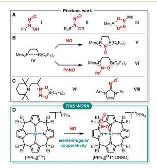
Fig. 1 (A–C) Previously reported reactivities of NO and nitrosobenzene with main-group element compounds. (D) Reactivity of calix[4]pyrrolato aluminate ( $[^{\text{Et}}1]^-$ ) with NO studied within this work. The asterisk in  $[^{\text{Et}}1^*-\text{ONNO}]^-$  indicates the dearomatization of one pyrrole unit.
