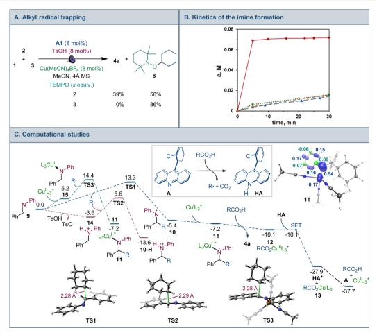
Fig. 3 (A) Mechanistic studies of the tricomponent amine construction. (B) Kinetic profile of imine 9 formation.  $-\bullet-$  with TsOH (8 mol%);  $-\bullet-$  with acid 3 (1 equiv.);  $-\bullet-$  with Cu(MeCN)<sub>4</sub>BF<sub>4</sub> (8 mol%);  $-\bullet-$  uncatalyzed reaction. (C) Computational studies of the radical amine formation,  $\Delta G$ , kcal mol<sup>-1</sup>, and the spin density isosurface (isovalue = 0.05) for intermediate 11. R = cyclohexyl, L = MeCN.
