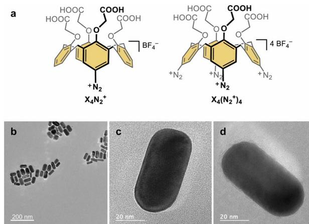
Fig. 1 (a) Structures of calix[4]arene mono-diazonium,  $X_4N_2^+$ , and calix[4]arene tetra-diazonium,  $X_4(N_2^+)_4$ , salts. TEM images of capped gold nanorods functionalized with (b) CTAB, (c)  $X_4N_2^+$ , and (d)  $X_4(N_2^+)_4$ .
