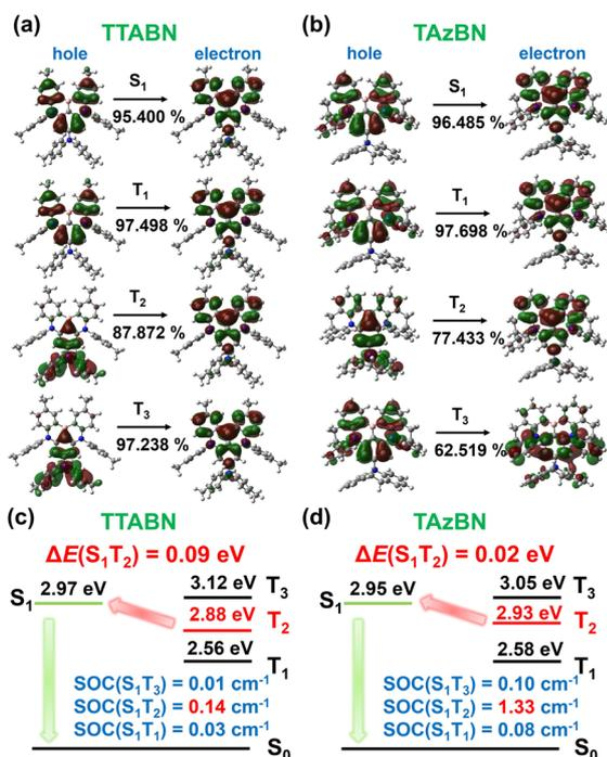
Fig. 2 Calculated natural transition orbitals (NTOs) based on the optimized  $S_0$  geometries, adiabatic excited state energies, and associated SOC matrix elements based on the optimized  $S_1$  geometries for (a and c) TTABN and (b and d) TAZBN, respectively, in toluene by TDA-DFT at the B3LYP/6-31G(d) level.
