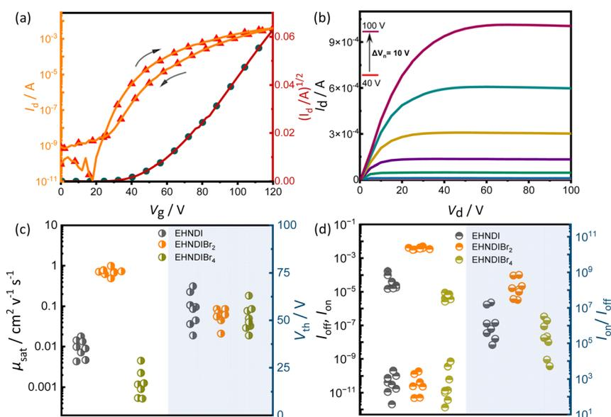
Fig. 3 OFET (a) transfer curve and (b) output curves for the EHNDIBr<sub>2</sub> thin film. (c)  $\mu_{sat}$  (left) and  $V_{th}$  (right) variations of EHNDI, EHNDIBr<sub>2</sub>, and EHNDIBr<sub>4</sub> devices. (d)  $I_{on}$  (top left),  $I_{off}$  (bottom left), and  $I_{on}/I_{off}$  (right) variations of EHNDI, EHNDIBr<sub>2</sub>, and EHNDIBr<sub>4</sub> devices.
