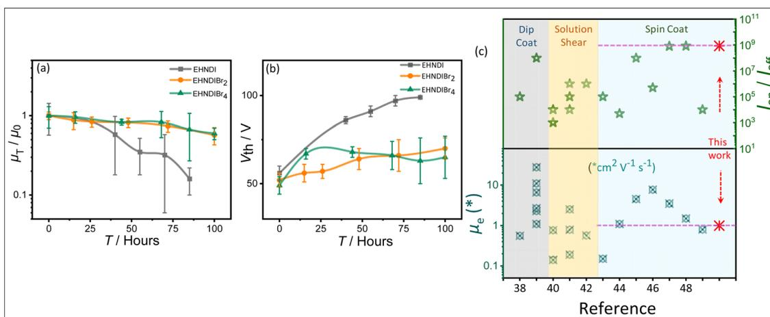
Fig. 4 Ambient stability measurement: (a) average saturation mobility change and (b) the threshold voltage changes ( $\Delta V_{\text{th}}$ ) with time of the OFET devices with exposure to the ambient atmosphere. (c) Summarized literature reports on the best device performances.<sup>38–49</sup> PVD processed and single crystal devices excluded.
