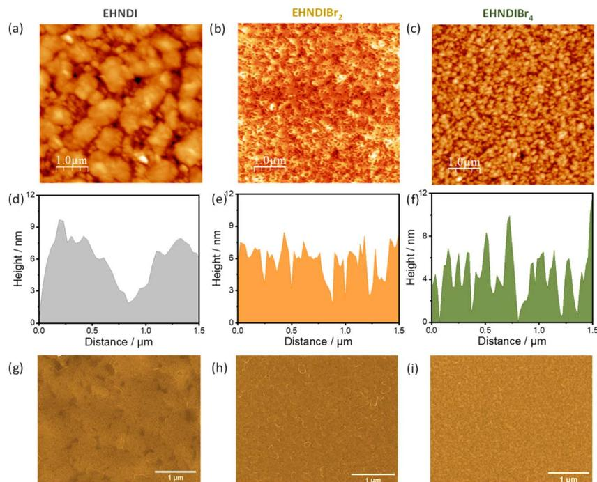
Fig. 7 AFM topography images, AFM height profiles and SEM images (a), (d), and (g) for EHNDI, (b), (e), and (h) for EHNDIBr<sub>2</sub> and (c), (f), and (i) for EHNDIBr<sub>4</sub> respectively.
