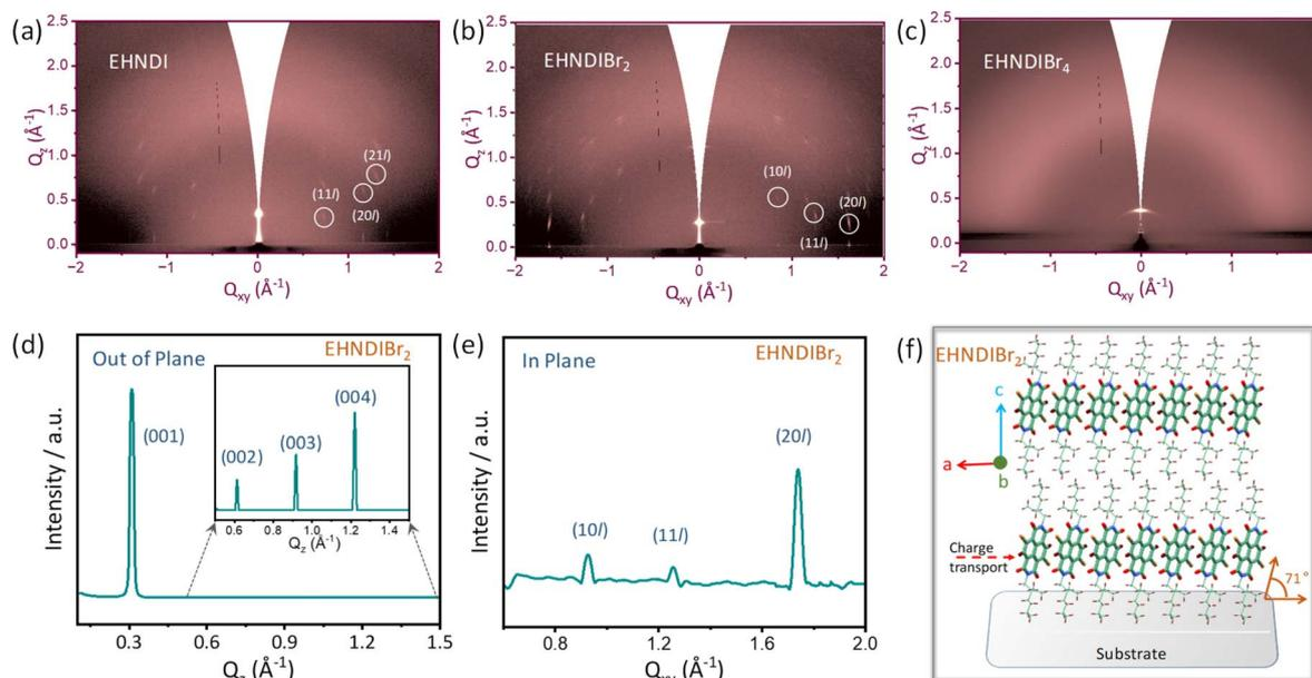
Fig. 6 (a–c) 2-D GIXRD diffraction profile of the optimized samples, (d) and (e) 1-D line cut profile of the EHNDIBr<sub>2</sub> films: (e) in-plane and (d) out-of-plane indicating periodic reflections of 001 planes. (f) Plausible molecular ordering on the surface.
