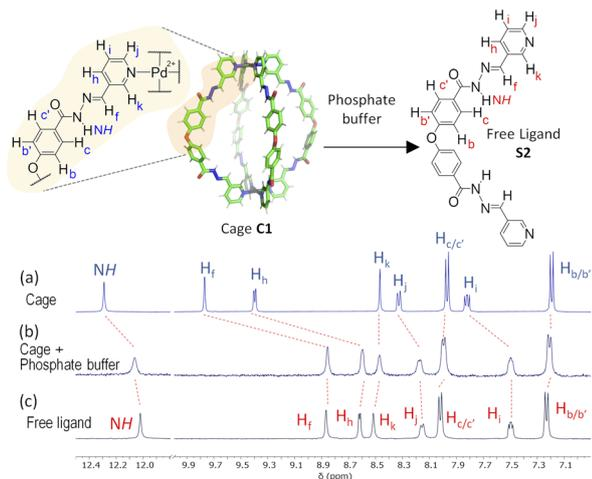
Fig. 6  $^1\text{H}$  NMR disassembly experiment of  $\text{C1}\cdot\text{NO}_3$  in  $\text{DMSO}-d_6$  (0.5 mM, 550  $\mu\text{L}$ ) with phosphate buffer (pH 7.2, 100 mM, 50  $\mu\text{L}$ ). (a)  $^1\text{H}$  NMR spectra of cage  $\text{C1}\cdot\text{NO}_3$ . (b)  $^1\text{H}$  NMR spectrum after the addition of phosphate buffer (ca. 5 min), causing cage disassembly. (c)  $^1\text{H}$  NMR spectra of free ligand (see structure S2 in ESI†).
