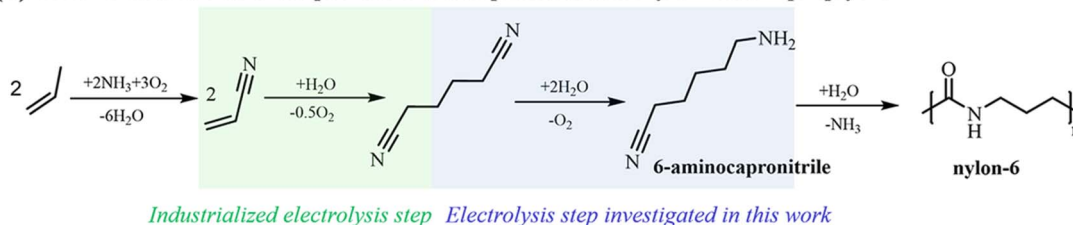
Fig. 1 Process steps for the formation of nylon-6 from (a) benzene and (b) propylene.
