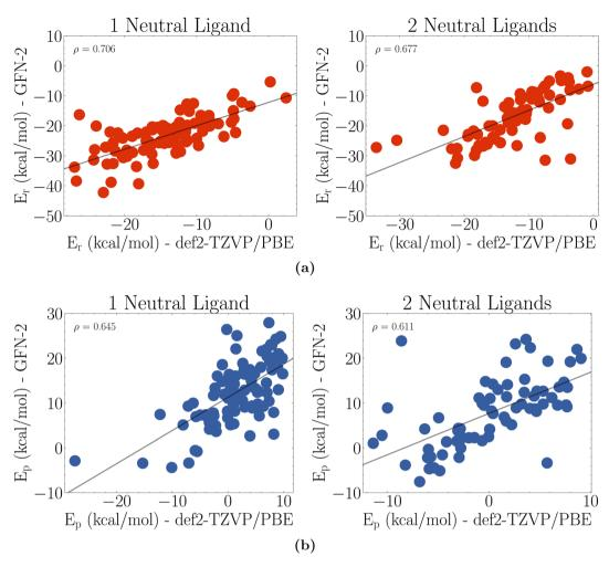
Fig. 5 Comparison of GFN2-xTB optimized reaction energies against def2-TZVP/PBE optimized reaction energies. (a) Reduction energies and (b) protonation energies. Here  $\rho$  is the Pearson correlation of the data.
