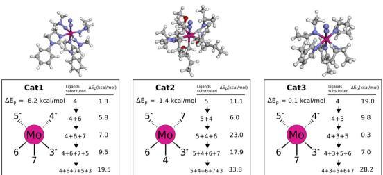
Fig. 12 Protonation energies for various ligand substitutions with  $NH_2^-$  and  $NH_3$  for Cat{1,2,3}. Energies are based on B3LYP single points of the def2-TZVP/PBE optimized  $Mo-N_2$  and  $Mo-N_2H^+$  intermediates. The orientation of the catalyst sketches in each box matches the 3D structure shown at the top.
