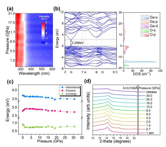
Fig. 3 (a) Pressure-dependent optical absorption spectra of the  $Ga_2O_3$  NCs. (b) DFT-calculated band structure and projected density of states of  $Ga_2O_3$  NCs under ambient conditions. (c) Absorption and emission energies of the  $Ga_2O_3$ NCs upon compression. (d) High-pressure ADXRD pattern for the  $Ga_2O_3$  NCs.
