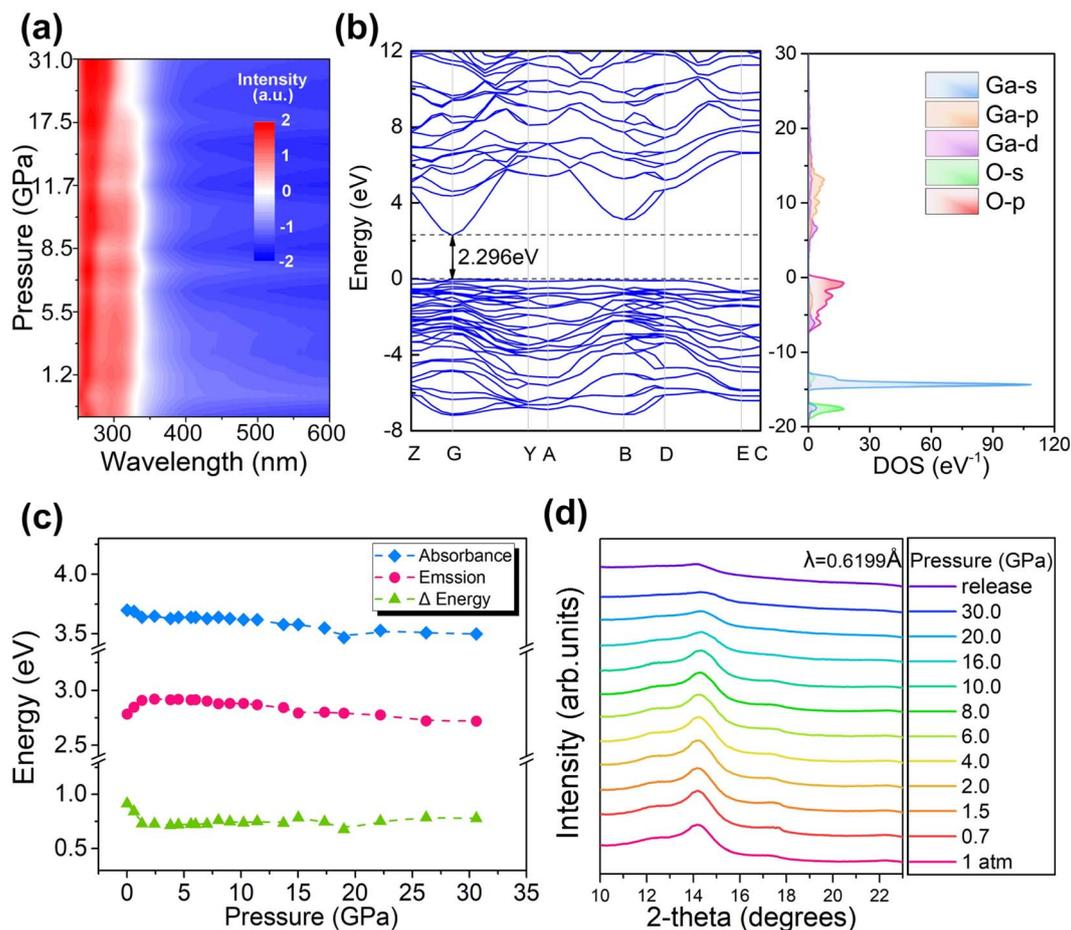
Fig. 3 (a) Pressure-dependent optical absorption spectra of the  $\text{Ga}_2\text{O}_3$  NCs. (b) DFT-calculated band structure and projected density of states of  $\text{Ga}_2\text{O}_3$  NCs under ambient conditions. (c) Absorption and emission energies of the  $\text{Ga}_2\text{O}_3$  NCs upon compression. (d) High-pressure ADXRD pattern for the  $\text{Ga}_2\text{O}_3$  NCs.
