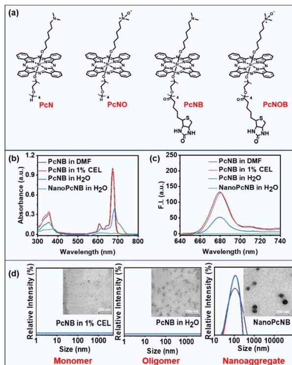
Fig. 2 (a) Chemical structure of the synthesized phthalocyanines. (b) Electronic absorption spectra of PcNB in DMF, water containing 1% CEL, pure water, and NanoPcNB in pure water. (c) Fluorescence emission spectra of PcNB in DMF, water containing 1% CEL, pure water, and NanoPcNB in pure water. (d) TEM imaging and DLS of PcNB in water containing 1% CEL (left), pure water (middle), and NanoPcNB in pure water (right), scale bar: 200 nm.
