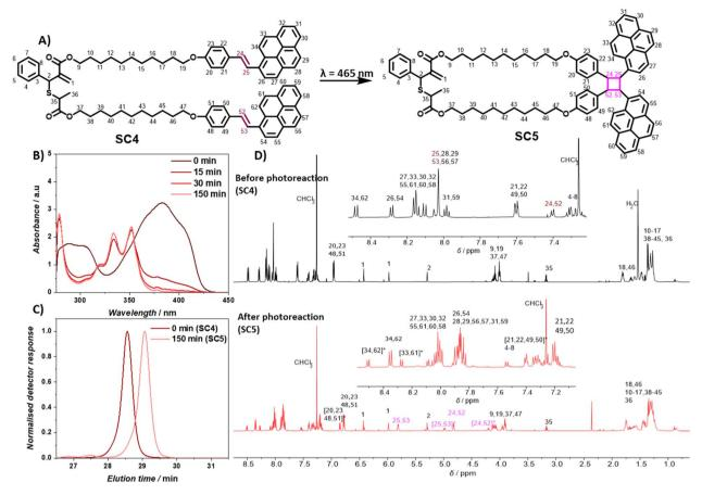
Fig. 1 Transformation from linear monomer SC4 to cyclic monomer SC5: (A) reaction; (B) absorption spectrum of reaction solution under  $\lambda$  = 465 nm irradiation (0.05 mg mL $^{-1}$  in THF); (C) SEC chromatogram of reaction solution (0.05 mg mL $^{-1}$  in THF) before photoreaction and after 150 min of  $\lambda$  = 465 nm irradiation; (D)  $^{1}$ H NMR of the monomer before and after irradiation showing the appearance of cyclobutane proton resonances after the irradiation.
