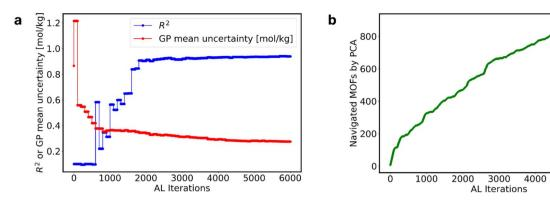
Fig. 4 Analysis of the GP-PCA model. (a) Evolution of average  $R^2$ , average GP MAE, and number of MOFs attained during 6000 iterations. (b) Number of MOFs navigated as a function of the number of iterations.
