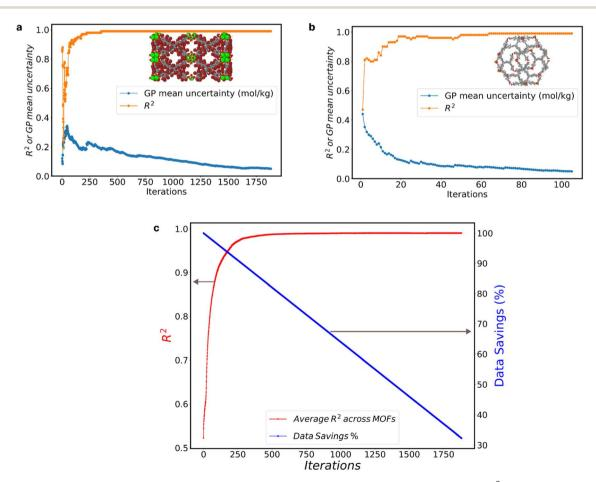
Fig. 2 Perfomance of GPR model across MOFs and data savings. (a) Evolution of the GP mean uncertainty and  $R^2$  of the MOF with the most AL iterations; (b) evolution of the GP mean uncertainty and  $R^2$  of the MOF with the fewest AL iterations; (c) average  $R^2$  across all MOFs (left *y*-axis) and the corresponding % data savings (right *y*-axis) at various AL iterations.
