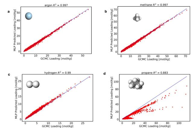
Fig. 3 Performance of the newly developed MLP model. The new MLP model was evaluated in the prediction of adsorption of real molecules among the range of alchemical training adsorbates (a) argon, (b) methane, and extrapolated outside the range of alchemical training adsorbates (c) hydrogen, and (d) propane.
