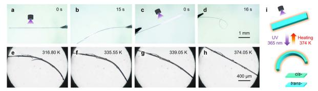
Fig. 3 Photomechanical deformation. (a-d) Acicular crystals of CTBB bend away from the light source upon irradiation on their (010) facet. (e-h) Recovery by heating of the shape of crystals that had been previously bent by exposure to light. (i) A schematic showing a simplified model of the photoinduced bending and thermally induced straightening of the crystal.
