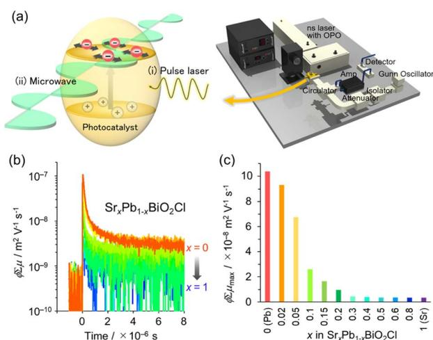
Fig. 8 (a) Schematic image of TRMC measurement. (b) TRMC transients of  $\text{Sr}_x\text{Pb}_{1-x}\text{BiO}_2\text{Cl}$  (orange for  $x = 0$  to blue for  $x = 1$ ). (c)  $\varphi\Sigma\mu$  maximum ( $\varphi\Sigma\mu_{\text{max}}$ ) values with respect to  $x$  for  $\lambda_{\text{ex}} = 266$  nm and  $I_0 = 6.8 \times 10^{15}$  photons  $\text{cm}^{-2}$  per pulse. (b and c) Adapted with permission from ref. 35 Copyright 2020, American Chemical Society.
