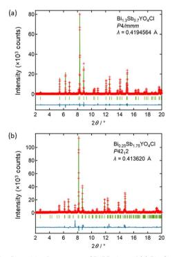
Fig. 5 The Rietveld refinement on SPXRD data of (a)  $Bi_{1.3}Sb_{0.7}YO_4Cl$ , assuming the  $Bi_2YO_4Cl$  (P4/mmm) model, and (b)  $Bi_{0.25}Sb_{1.75}YO_4Cl$ , assuming the  $Sb_2YO_4Cl$  ( $P42_12$ ) model. The red markers, the green solid line, and the blue solid line represent observed, calculated and difference intensities, respectively. The green ticks indicate the calculated Bragg reflections.
