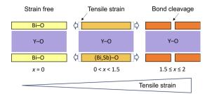
Fig. 2 Schematic illustration showing 'tensile strain' by Sb substitution in  $Bi_2YO_4Cl$ . With the Sb substitution of Bi, tensile strain is imposed from the inner  $YO_2$  sublayer (blue) to the outer (Bi,Sb)O sublayer within the (Bi,Sb) $_2YO_4$  triple fluorite slab, eventually leading to a phase transition with bond-cleaved  $Sb_2YO_4Cl$ -type structure.
