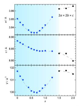
Fig. 4 The x dependence of the lattice parameters in  $Bi_{2-x}Sb_xYO_4Cl$  ( $0 \le x \le 2$ ): (top) a-axis, (middle) c-axis, and (bottom) volume. For  $1.5 \le x \le 2$ , the a-axis and volume are normalized to the ideal P4/mmm unit cell.
