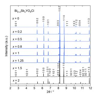
Fig. 3 Room temperature SPXRD patterns of  $Bi_{2-x}Sb_xYO_4Cl$  ( $0 \le x \le 2$ ). The samples with  $x \le 1.25$  are indexed with the P4/mmm space group ( $Bi_2YO_4Cl$  structure). Peaks are indexed based on the ideal tetragonal structure of  $Bi_2YO_4Cl$ . See Fig. S2† showing the absence of superlattice peaks for  $x \le 1.25$ . The data was collected at a wavelength of  $\lambda = 0.41946$  Å ( $x \le 1$ ) or 0.41362 Å ( $x \le 1$ ).
