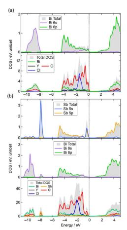
Fig. 9 (a) Density of states (DOS) of  $\rm Bi_2YO_4Cl$  and partial DOS (PDOS) for Bi 6s and Bi 6p states. (b) DOS of  $\rm Bi_{1.5}Sb_{0.5}YO_4Cl$  and PDOS for Sb and Bi.
