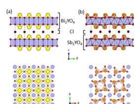
Fig. 1 The crystal structures of (a)  $Bi_2YO_4Cl^{28}$  and (b)  $Sb_2YO_4Cl^{29}$  with triple fluorite slabs, viewed along the [100] direction (top) and the [001] direction (bottom). Yellow, orange, blue, red, and brown spheres indicate Bi, Sb, Y, O and Cl atoms, respectively. Broken lines represent the unit cell. Bi/Sb–O bonds with negligible bond valence (<0.1) are not drawn (Table S5†).
