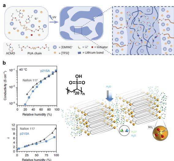
Fig. 14 (a) A tough ionogel with high ionic conductivity promoted by lithium ions. Copyright 2023, Wiley-VCH. Reproduced with permission from ref. 132. (b) Layered sulfonated polyethylene with well-controlled methylene chain segment folding for crystallization and highly uniform hydrated acid layers for high proton conductivity. Copyright 2018, Springer Nature. Reproduced with permission from ref. 133.
