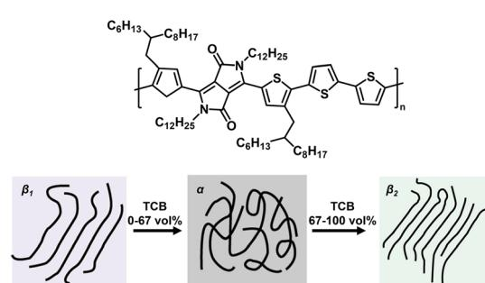
Fig. 4 The gradual  $\beta_1$ - $\alpha$ - $\beta_2$  phase transition of D-PDPP4T-HD by adding TCB into CF from 0 vol% to 100 vol%. Copyright 2019, Springer Nature. Reproduced with permission from ref. 43.
