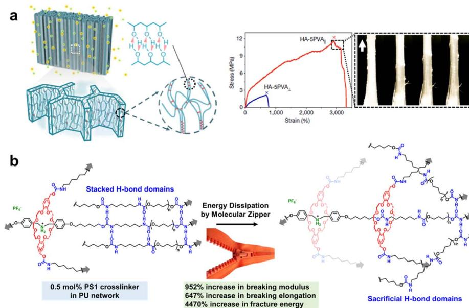
Fig. 11 (a) A multi-length-scale hierarchical hydrogel architecture toughened *via* a freezing-assisted salting-out synergic treatment. Copyright 2021, Springer Nature. Reproduced with permission from ref. 106. (b) A H-bond-crosslinked PU elastomer toughened by a molecular zipper strategy. Copyright 2020, Wiley-VCH. Reproduced with permission from ref. 107.
