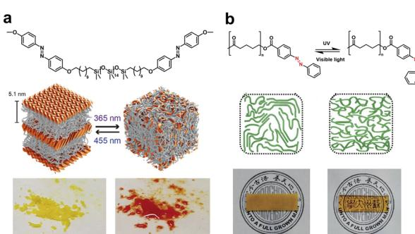
Fig. 5 (a) Isomerism induced solid–liquid transition of azo-functionalized siloxane oligomers under UV/vis irradiation. Copyright 2018, Wiley-VCH. Reproduced with permission from ref. 49. (b) Photo-switchable  $T_m$  and transparency of azo-terminated PCL. Copyright 2021, Royal Society of Chemistry. Reproduced with permission from ref. 50.
