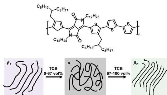
Fig. 4 The gradual  $\beta_1$ - $\alpha$ - $\beta_2$  phase transition of D-PDPP4T-HD by adding TC into CF from 0 vol% to 100 vol%. Copyright 2019, Springer Nature. Reproduced with permission from ref. 43.
