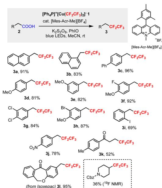
**Scheme 4** Scope of decarboxylative pentafluoroethylation using **1**.<sup>a</sup> <sup>a</sup>General conditions: **1** (0.2 mmol), **2** (0.4 mmol),  $[\text{Mes-Acr-Me}][\text{BF}_4]$  (3 mol%),  $\text{K}_2\text{S}_2\text{O}_8$  (0.4 mmol), PhIO (0.2 mmol), MeCN (2.0 mL), blue LEDs, rt for 12 h under argon. Isolated yields based on **1**.
