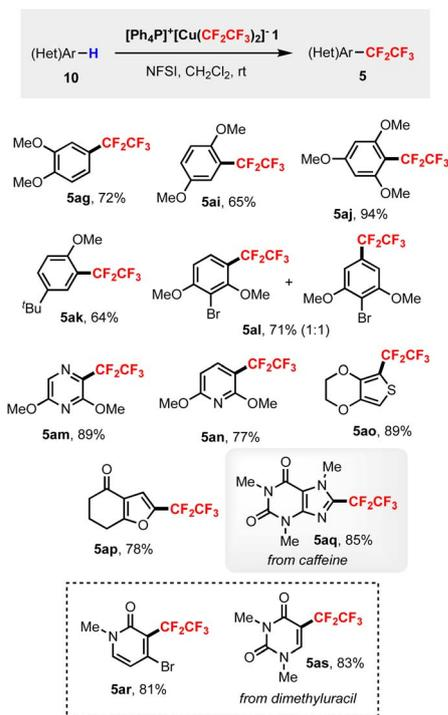
**Scheme 8** Oxidative pentafluoroethylation of (hetero)aromatic C–H bond using **1**.<sup>a</sup> General conditions: **1** (0.2 mmol), **10** (1.0 mmol), NFSI (0.6 mmol), CH<sub>2</sub>Cl<sub>2</sub> (2.0 mL), under argon, 12 h. Isolated yields.
