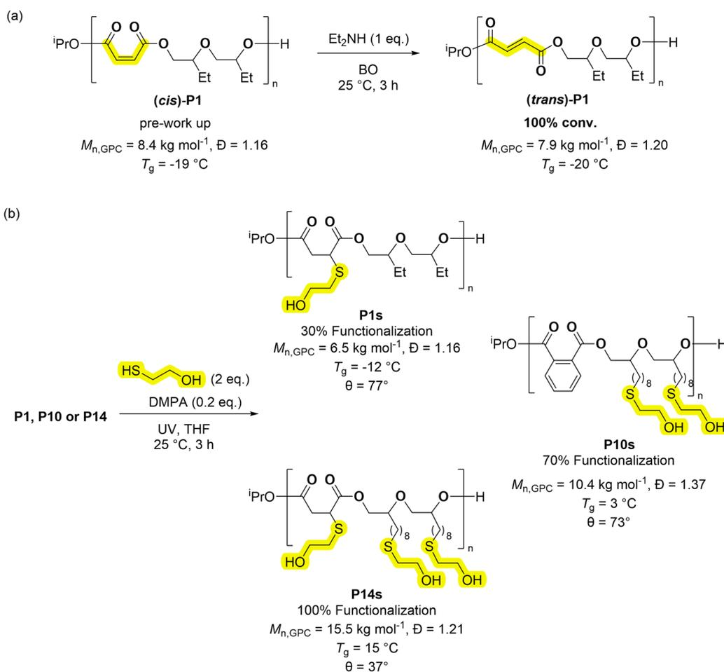
**Scheme 3** Post-copolymerisation functionalization of poly(ester-*alt*-ethers) (ABB). (a) Isomerization of the alkene moieties in **P1**; (b) processes to install hydroxyl groups, using thiol-ene reactions, onto the polymer repeat units. These apply the copolymers, **P1**, **P10**, **P14**, to achieve 30, 70 and 100% hydroxyl substitution, respectively (where % refers to the extent of hydroxyl substitution of both A and B repeat units). Note that the thiol-ene reactions are regio-random.
