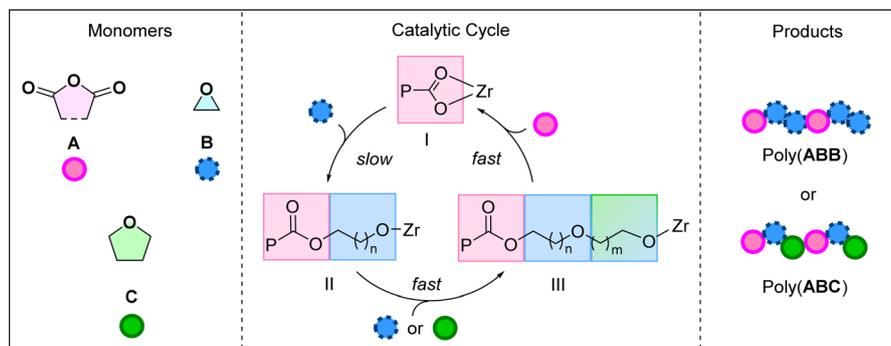
**Scheme 1** Left: Monomers used within this work, Middle: catalytic cycles for anhydride/cyclic ether ring-opening copolymerisation (ROCOP), Right: **ABB** or **ABC** poly(ester-*alt*-ethers) formed by the Zr(IV) catalyst, P: polymeryl chain; Zr: metal active site. All monomers/polymers represented by simplest substitution pattern.
