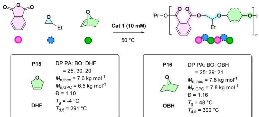
**Scheme 2** Ring-opening copolymerisation (ROCOP) of PA, BO and cyclic ethers with catalyst **1**. ROCOP conditions for **P15**: [1] = 10 mM, [PA] = 0.5 M, BO = 0.25 mL, 2.8 M, DHF = 0.75 mL, 9.9 M, total volume of BO + OBH = 1 mL, 50 °C. ROCOP conditions for **P16**: [1] = 10 mM, [PA] = 0.5 M, BO = 0.25 mL, 2.8 M, OBH = 0.75 mL, 7.4 M, total volume of BO + OBH = 1 mL, 50 °C.
