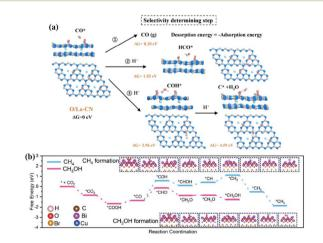
Fig. 7 (a) Calculated free energy for the photocatalytic  $CO_2$  reduction reaction of the selectivity-determining step. This figure has been reproduced from ref. 67 with permission from American Chemical Society, copyright 2020. (b) The DFT-calculated free energy diagram for the hydrogenation of  $CO_2$  to  $CH_3OH$  and  $CH_4$  over  $Cu_1@BiOBr$ . This figure has been reproduced from ref. 68 with permission from Wiley-VCH, copyright 2023.
