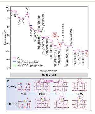
Fig. 2 (a) Gibbs free energy diagrams of  $CO_2$  reduction on the  $Cu-Ti-V_O$  unit. This figure has been reproduced from ref. 46 with permission from Springer Nature, copyright 2023. (b) The C-C coupling process of  $Ov-WO_3$  and  $S-Ov-WO_3$ . This figure has been reproduced from ref. 47 with permission from Elsevier, copyright 2023.
