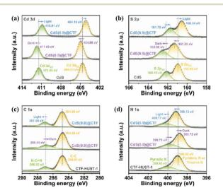
Fig. 12 High-resolution XPS spectra of (a) Cd 3d, (b) S 2p, (c) C 1s, and (d) N 1s of CdS, CTF-HUST-1, and CdS(0.9)@CTF samples. The  $in\ situ$  XPS measurement was performed under light irradiation. These figures have been reproduced from ref. 138 with permission from Wiley-VCH, copyright 2023.
