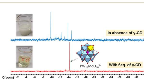
Fig. 6  $^{31}\text{P}$  NMR spectra of the supernatant solutions resulting from the addition of cationic  $\text{MoO}_2^{2+}$  species (1.2 eq. per monovacant POM) into a solution of  $\text{PW}_{11}\text{O}_{39}^{7-}$  containing no  $\gamma$ -CD or six equivalents of  $\gamma$ -CD. The final pH of both solutions was 0.6.
