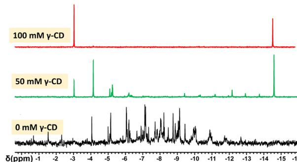
Fig. 5  $^{31}P$  NMR spectrum of 24 h aged aqueous solutions in which  $PW_{12}O_{40}^{3-}$  (25 mM),  $PMo_{12}O_{40}^{3-}$  (25 mM), and various amounts of  $\gamma$ -CD (from 0 to 100 mM) have been introduced.
