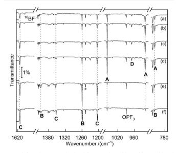
Fig. 1 Infrared spectra obtained from codeposition of laser-ablated  $^{10}$ B-enriched boron atoms with 0.05% PF $_3$  in solid neon matrices after (a) 60 min of sample deposition at 5 K, (b) 9 K annealing, (c) 10 min of 470 nm irradiation, (d) 10 min of 455 nm irradiation, (e) 15 min of > 220 nm irradiation, (f) 11 K annealing. A: B=PF $_3$ , B: F $_2$ B-PF (tentatively), C: F $_2$ B-P=BF, D: F $_3$ P-B=B-PF $_3$  (tentatively), unassigned bands are marked with asterisks.
