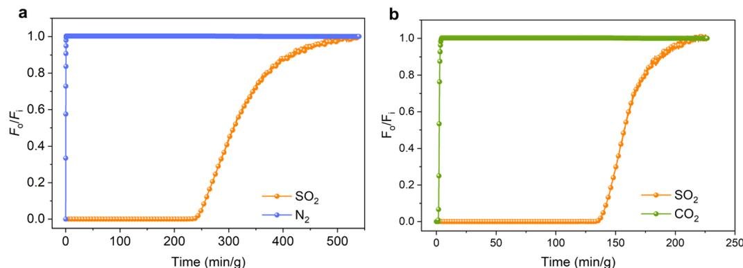
Fig. 3 Separation of  $\text{SO}_2$ ,  $\text{N}_2$  and  $\text{CO}_2$  by HIAM-330: breakthrough plots for (a) the  $\text{SO}_2/\text{N}_2$  mixture (2500 ppm  $\text{SO}_2$ , 75%  $\text{N}_2$  in He, and total flow rate:  $20 \text{ mL min}^{-1}$ ) and (b) the  $\text{SO}_2/\text{CO}_2$  mixture (2500 ppm  $\text{SO}_2$ , 15%  $\text{CO}_2$  in He, and total flow rate:  $20 \text{ mL min}^{-1}$ ) in HIAM-330 at 298 K.
