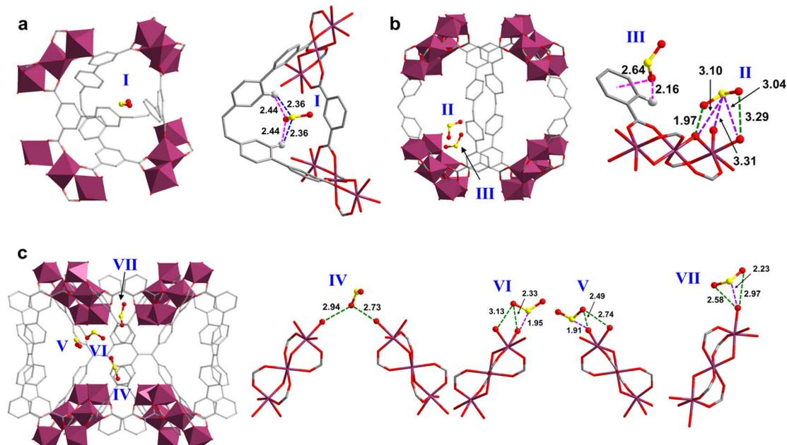
Fig. 4 Adsorption domains of  $\text{SO}_2$  in HIAM-330 determined by Rietveld refinements of high-resolution *in situ* synchrotron powder X-ray diffraction. (a) site I, (b) sites II and III, (c) sites IV–VII.
