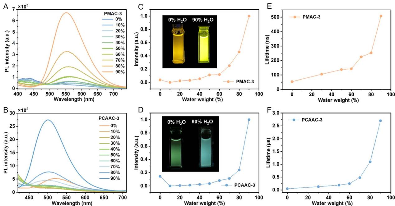
Fig. 4 (A) **PMAC-3** and (B) **PCAAC-3** in THF/water mixtures with different water fractions ( $f_w$ ) under 380 nm and 370 nm excitation. Emission intensity vs.  $f_w$  of (C) **PMAC-3** and (D) **PCAAC-3**. Inset: photos in THF/water mixtures ( $f_w = 0$  and 90%) under 365 nm excitation. Lifetimes vs.  $f_w$  of (E) **PMAC-3** and (F) **PCAAC-3**.
