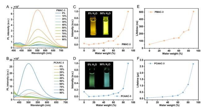
Fig. 4 (A) PMAC-3 and (B) PCAAC-3 in THF/water mixtures with different water fractions ( $f_w$ ) under 380 nm and 370 nm excitation. Emission intensity vs.  $f_w$  of (C) PMAC-3 and (D) PCAAC-3. Inset: photos in THF/water mixtures ( $f_w = 0$  and 90%) under 365 nm excitation. Lifetimes vs.  $f_w$  of (E) PMAC-3 and (F) PCAAC-3.
