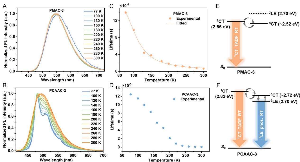
Fig. 3 Normalized PL spectra of (A) **PMAC-3** and (B) **PCAAC-3** under 375 nm excitation at different temperatures from 77 to 300 K. (C) Fitting line of the temperature-dependent lifetime data from 77 to 300 K (symbols) according to eqn (S1)† (line) of **PMAC-3**. (D) Temperature-dependent lifetime data from 77 to 300 K of **PCAAC-3**. Schematic energy diagrams of the relevant states for (E) **PMAC-3** and (F) **PCAAC-3**.
