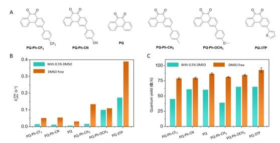
Fig. 2 Overview of the first order reaction rate ( $k_{\rm obs}$ ) and photoreaction quantum yield ( $\Phi_{\rm P}$ ) of the PQ-ERA photoclick reaction system. (A) Structures of the investigated PQs; (B) The  $k_{\rm obs}$ (390) and (C)  $\Phi_{\rm P}$  of PQ-ERA photoclick reaction. Cyan: with DMSO, orange: DMSO-free, respectively. NB:  $k_{\rm obs}$  and  $\Phi_{\rm P}$  are measured under different conditions (for more detailed information see ESI,† Section 2.1 and 2.2).
