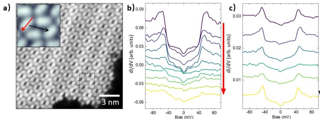
Fig. 1 STM topograph and spectroscopy of CTPO molecules on the Au(111) surface with tunneling conditions  $(-0.2$  V, 20 pA). Inset is the enlarged image of the area marked with a dashed box on the image. (b) and (c)  $dI/dV$  tunneling spectra taken in the monolayer, along red and black arrows depicted in (a). The spectra are offset for clarity. All the spectra were acquired with equal spacing along two lines at a set point  $(-0.1$  V, 0.1 nA) with feedback off.
