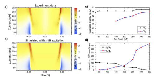
Fig. 5 Influence of tunneling distance on the tunneling spectra. (a) Experimental tunneling spectra under different set points. (b) Simulated tunneling spectra with the three-channel model. Dashed curves are guides for the peak shift. (c) Fitted values of threshold voltages  $V_1$  and  $V_2$ . (d) Normalized coupling coefficients at different set points.
