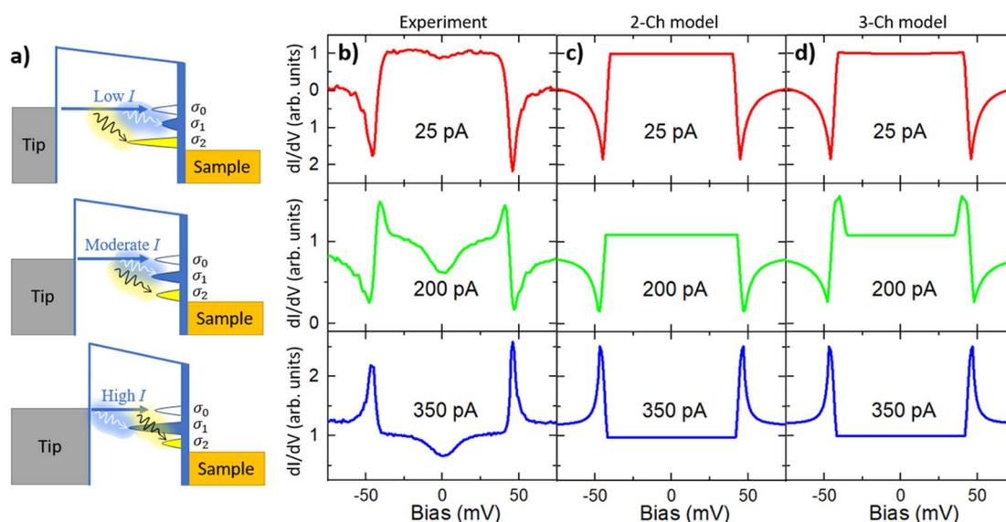
Fig. 4 Multi-channel model and the differential tunneling spectra. (a) Diagram of three-channel model at different tunneling distances. (b–d) Experimental  $dI/dV$  spectra and simulation with the two-channel model and three-channel model, respectively.
