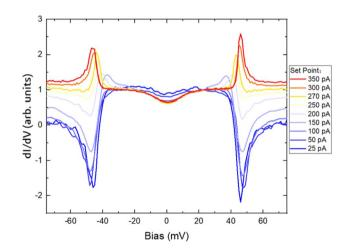
Fig. 3 Normalized dI/dV spectra taken on a single molecule with various tunneling junction distances. The tunneling set point was changed from 25 pA to 350 pA, with the bias voltage set as -0.1 V.
