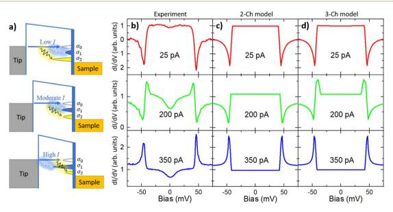
Fig. 4 Multi-channel model and the differential tunneling spectra. (a) Diagram of three-channel model at different tunneling distances. (b–d) Experimental dI/dV spectra and simulation with the two-channel model and three-channel model, respectively.
