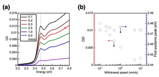
Fig. 2 a) Absorbance spectra of perovskite quantum dot (PeQD) monolayer prepared with different withdrawal speeds. (b) Dependence of withdrawal speed on the optical density (OD) and first excitonic peak position of the PeQD monolayer.
