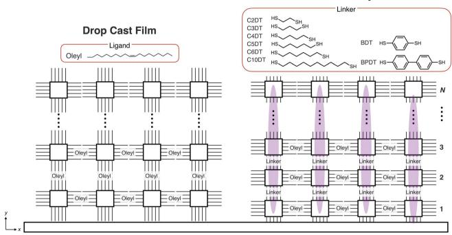
Fig. 1 Schematic illustration of layer-by-layer (LbL) assembly of perovskite quantum dots (PeQDs) and coupling strength controlled by inter-PeQD distance with different linker lengths.
