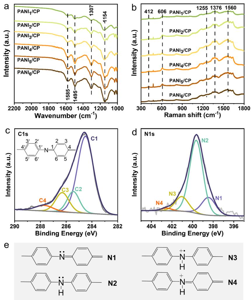
Fig. 2 Chemical structure characterization. (a) FT-IR and (b) Raman spectra of PANI/CP samples. (c) Deconvoluted C 1s XPS and (d) N 1s XPS spectra of PANI<sub>1</sub>/CP samples. (e) Structures of four nitrogen species.
