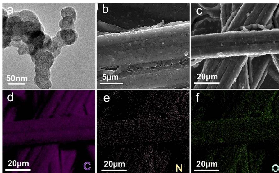
Fig. 1 Microscopic morphology characterization. (a) TEM (b) and (c) SEM images of PANI<sub>1</sub>/CP. SEM-EDAX images of (d) C element, (e) N element and (f) O element of the PANI<sub>1</sub>/CP surface.
