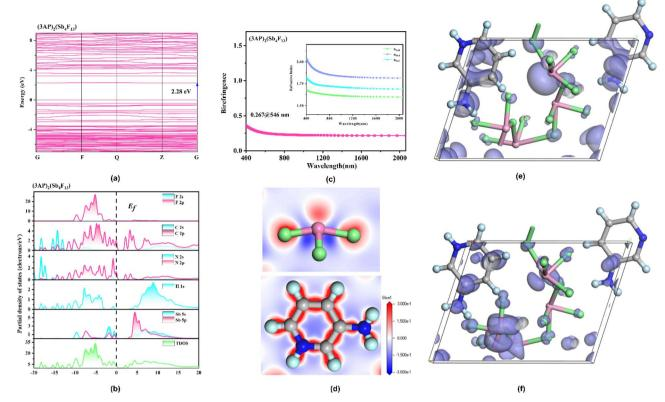
Fig. 8 Calculated band structure (a), total and partial densities of states (b), birefringence (c), electron density difference maps (d) and SHG density of  $d_{22}$  in the VB (e) and the CB (f) for  $(3AP)_2(Sb_4F_{13})$ .
