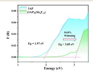
Fig. 5 The experimental bandgap spectra of 3AP and  $(3AP)_2(Sb_4F_{13})$ .
