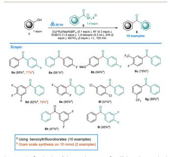
**Scheme 3** Synthesis of benzophenones 6 utilizing the method developed.
