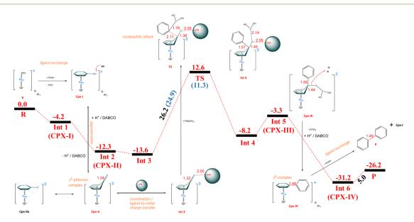
Scheme 4 Proposed plausible mechanism of the title transformation with boronic acids including DFT energy profile for Ru-catalysed formal activation of Ph-OH bond, transformed to biphenyl. All the reported energy values are presented in kcal  $mol^{-1}$  with reference initial reactant (R) at 0.0 kcal  $mol^{-1}$  at B3LYP/Def2TZVPP level of theory. Measured bond lengths are reported in Angstroms (Å). Values in blue color present dispersion corrected energies at B3LYP-D3 functional.
