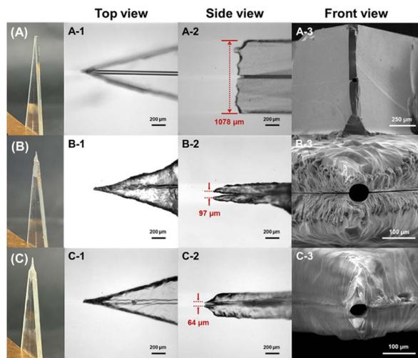
**Fig. 2** Photographs of 3D nESI emitters monolithically integrated on glass microfluidic chips (A) before etching and after etching for 15 min (B) without and (C) with continuous fluid. A-1, B-1 and C-1 are top views of nESI emitters; A-2, B-2 and C-2 are side views of nESI emitters; A-3, B-3 and C-3 are scanning electron microscopy (SEM) images of nESI emitter tips.
