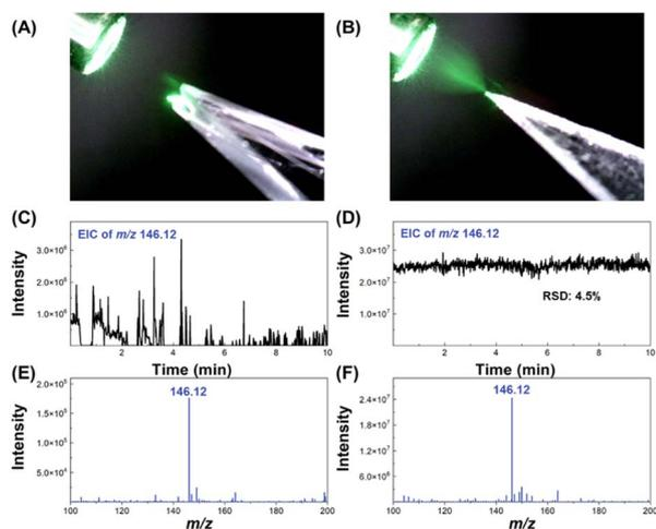
Fig. 3 The electrospray plume of (A) an unetched 2D nESI emitter and (B) an etched 3D nESI emitter. The EIC of ACh ( $m/z$  146.12) was obtained from (C) an unetched 2D nESI emitter and (D) an etched 3D nESI emitter. Mass spectra were obtained from (E) an unetched 2D nESI emitter and (F) an etched 3D nESI emitter. The solvent used was methanol–water 50 : 50 containing 1% formic acid (FA); the flow rate was  $500 \text{ nL min}^{-1}$ ; the applied nESI voltage was +4000 V.
